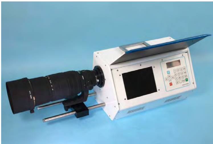
The Specialised Imaging SIRII ballistic range camera. 4000 by 3000 pixels, 20ns exposure.
