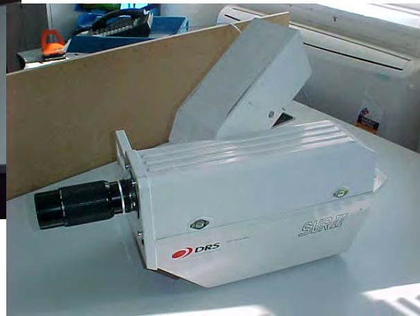
Pictures show the Hadland SVR2 ballistic range camera
