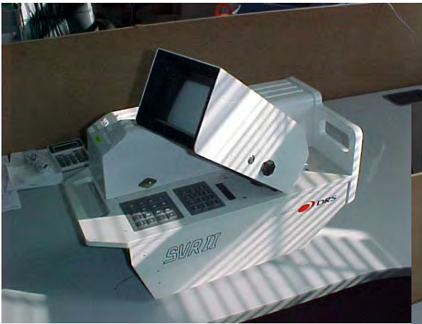
Pictures show the Hadland SVR2 ballistic range camera
