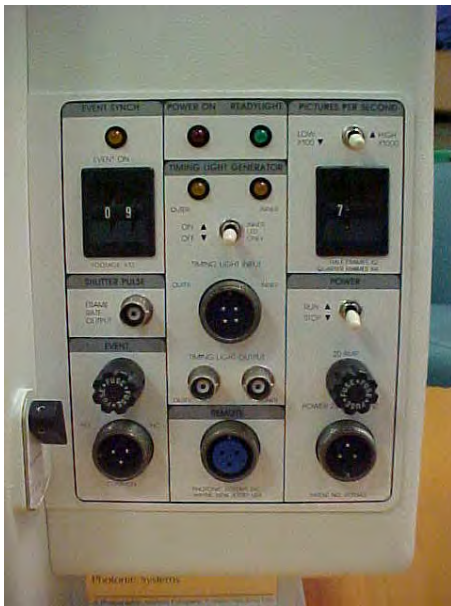
The Hadland Hyspeed was capable of 10000 frames per second full-height, 40000 ¼ height
