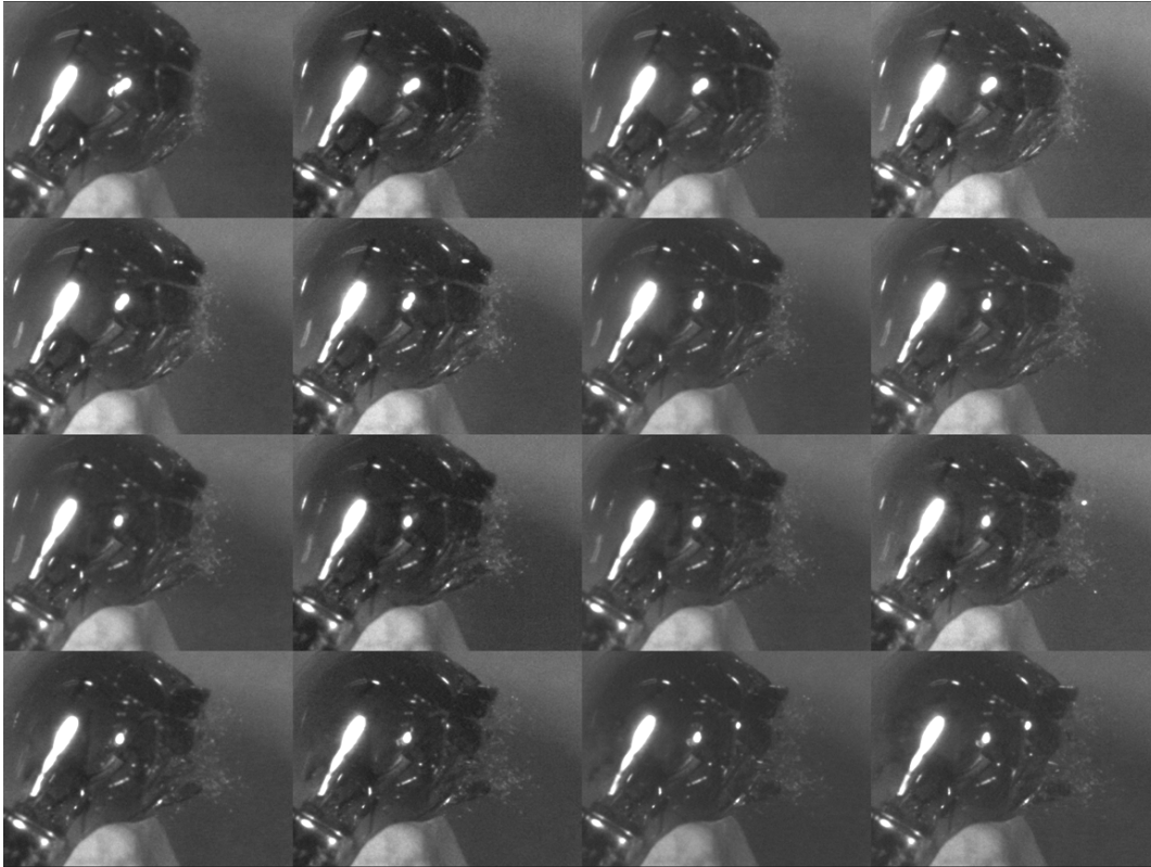
16-frame sequence of pellet impacting a small bulb
